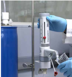
Remote Dispensing System for Drum Dispensing
