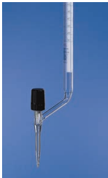
Burettes, BLAUBRAND®, class AS, Boro 3.3, DE-M, lateral valve cock, blue Schellbach stripe
